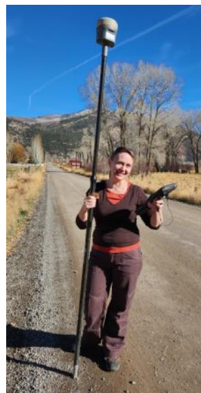
While doing a survey, Mona uses a controller (on the right) and a rover/base (on the left) for taking GPS locations in the field.
