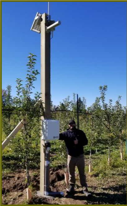
John Miller next to a research quality advanced soil moisture monitoring system that he installed in 2018
